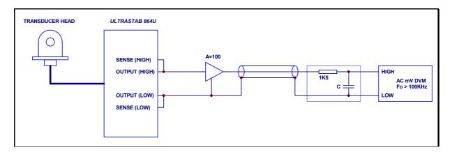
The filtering technique can also be used to limit the bandwidth of the 864U in applications, where a more narrow bandwidth is acceptable and a lower noise figure is desirable.
