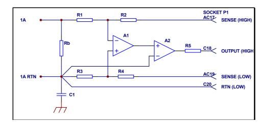
In order to obtain the highest performance from the *ULTRASTAB 864U* the output circuitry is designed as a 4 terminal system.
