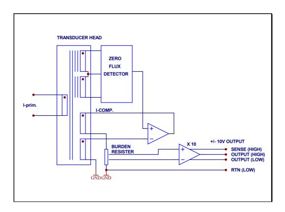
A very sensitive detector circuit will detect, when zero flux is obtained, and an analog 0 to  $\pm 10$ V signal will be generated at the output terminals in a direct 0 to 100% proportion to the primary current.
