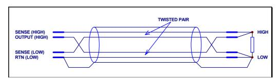
As an example a wire, 2.3 metres long with a cross section of 0.5 square mm will have a resistance of 87 m $\Omega$ . This will alter R2 by 0.087 / 10.000 = 8.7 ppm.
